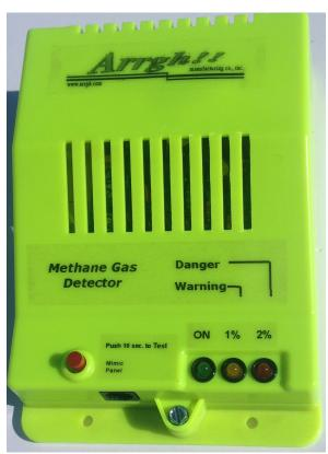
he Methane gas detector protects rooms and other locations where Methane gas can accumulate by monitoring gas levels. Concentrations of 5% to 15% mixed with air can be explosive. Sparks or hot surfaces can ignite them. The Methane gas detector will provide a warning and facilitate dissipation of the Methane, by operating alarms and exhaust fans before it reaches the lower explosive limit of 5%.
